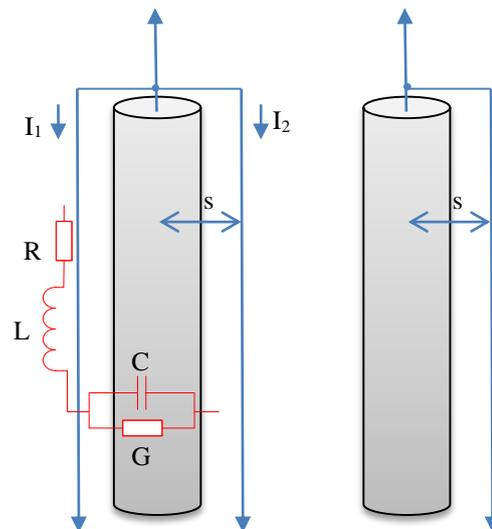
Fig. 1. Symmetrical and asymmetrical down-conductors.
