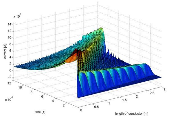
Fig. 2. Current distribution in one down-conductor of the length of 3 m when the input impulse  $10/350 \mu s$  and  $I_1=150$  kA.
