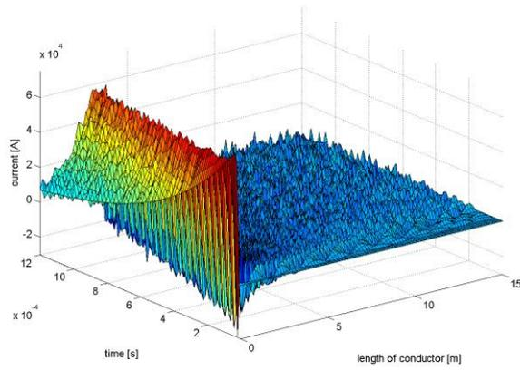
Fig. 4. Current distribution in one down-conductor of the length of 15 m when the input impulse 10/350  $\mu$ s and  $I_1=150$  kA.
