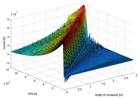
Fig. 6. Current distribution in both down-conductors of the length of 3 m when the input impulse 10/350  $\mu$ s and  $I_1=75$  kA.
