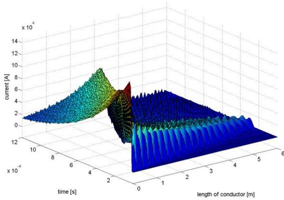
Fig. 3. Current distribution in one down-conductor of the length of 6 m when the input impulse 10/350  $\mu$ s and  $I_1=150$  kA.
