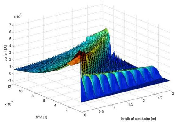
Fig. 5. Current distribution in one down-conductor of the length 3 m when the input impulse 10/350  $\mu$ s and  $I_1=75$  kA.
